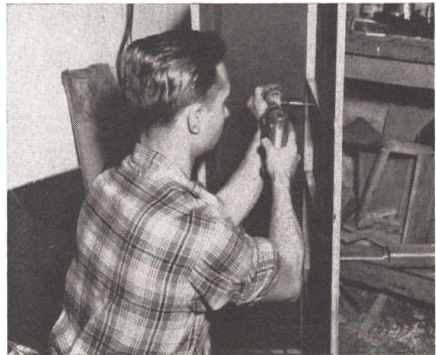
Specialized shop operations are made easy with low-priced power-tool attachments like this angle head.
