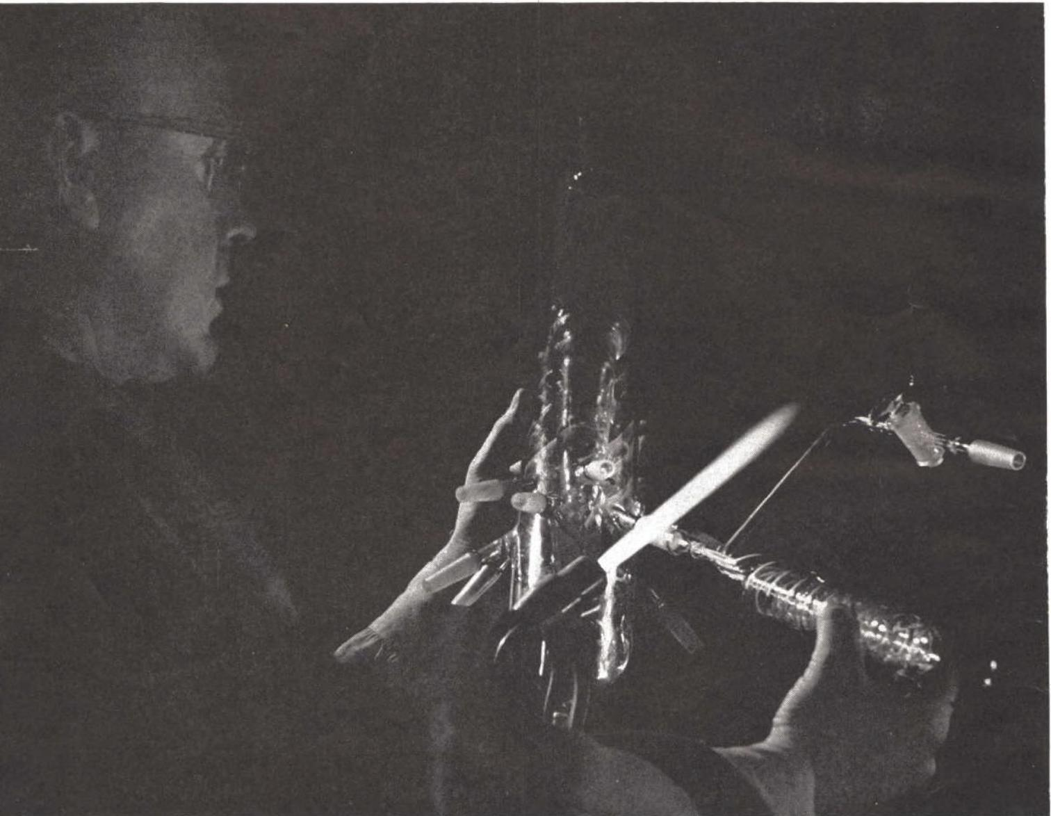
Tracerlab glass blower fashions highly intricate tube combination which will be used in Carbon-14 work.
